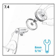
Mount M1 can be used to attach NUVIZ Controller to a handlebar
