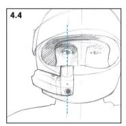
Align the center of the NUVIZ display with your right eye for optimal position
