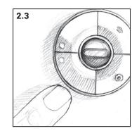
Press any key to power on and activate the Controller
