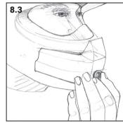
Press the plastic lens collar to adjust the view as desired
