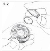
Insert the battery (CR2032) with the ,"+" sign facing up as indicated on the Controller
