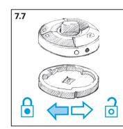
Note the lock/unlock symbols when attaching or removing the Controller
