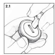
Open the battery cover of the Controller with the tool provided
